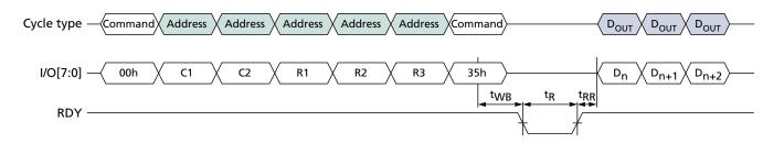
Figure 49: READ FOR INTERNAL DATA MOVE (00h-35h) with RANDOM DATA READ (05h-E0h)
