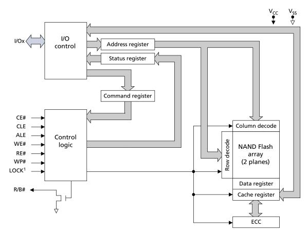
Note: 1. The LOCK pin is used on the 1.8V device.
