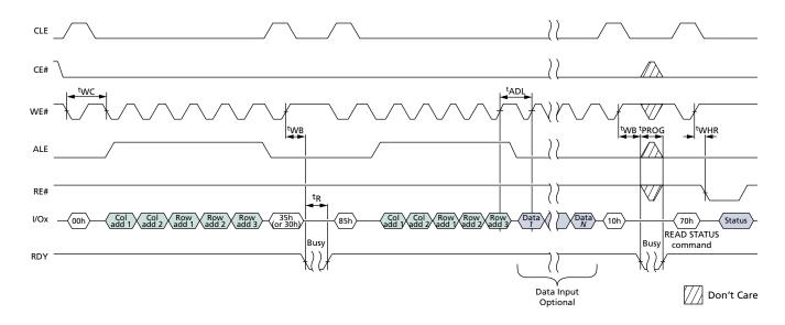
Figure 96: INTERNAL DATA MOVE (85h-10h) with Internal ECC Enabled
