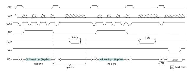
Figure 77: TWO-PLANE/MULTIPLE-DIE READ STATUS Cycle
