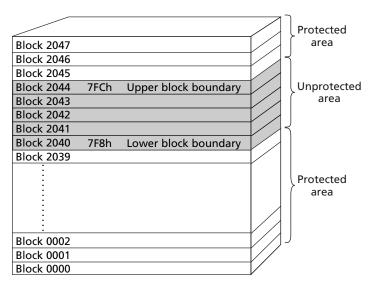
Figure 56: Flash Array Protected: Invert Area Bit = 1
