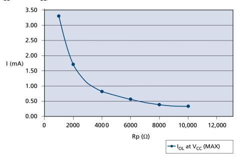
Figure 20: I<sub>OL</sub> vs. Rp (1.8V V<sub>CC</sub>)
