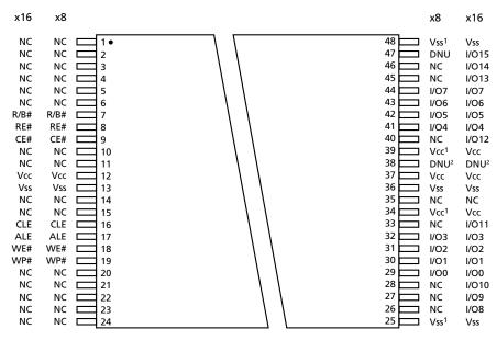
Notes: 1. These pins might not be bonded in the package; however, Micron recommends that the customer connect these pins to the designated external sources for ONFI compatibility.
