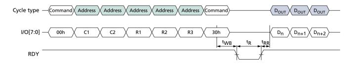
Figure 37: READ PAGE (00h-30h) Operation with Internal ECC Enabled
