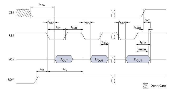
Figure 15: Asynchronous Data Output Cycles (EDO Mode)
